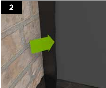
At the host wall fold the vertical DPC over the top of the membrane prior to battening out.
